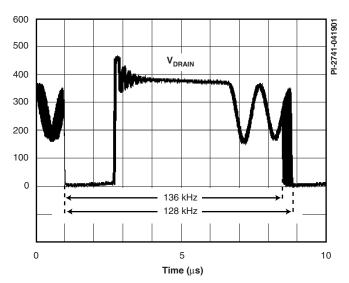
Figure 4. Frequency Jitter.
