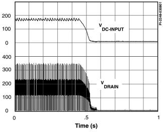
Figure 12. Normal Power-down Timing (without UV).
