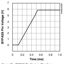
Figure 26. BYPASS Pin Start-up Waveform.
