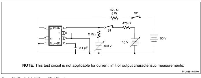
Figure 18. TinySwitch-II General Test Circuit.
