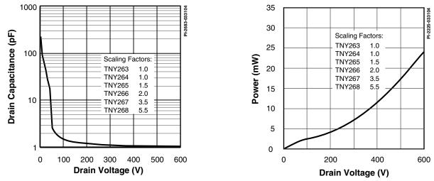
Figure 28. Coss vs. Drain Voltage.
