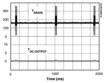
Figure 5. TinySwitch-II Auto-Restart Operation.
