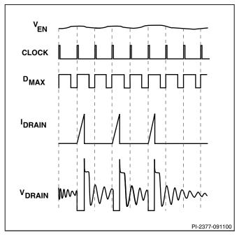
Figure 8. TinySwitch-II Operation at Medium Loading.
