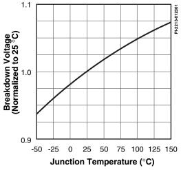
Figure 22. Breakdown vs. Temperature.
