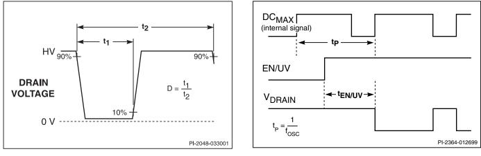
Figure 19. TinySwitch-II Duty Cycle Measurement.
