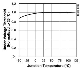
Figure 30. Under-voltage Threshold vs. Temperature.
