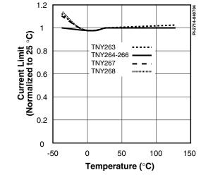
Figure 24. Current Limit vs. Temperature.
