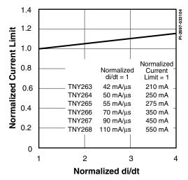
Figure 25. Current Limit vs. di/dt.
