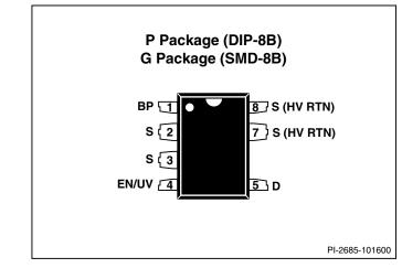
Figure 3. Pin Configuration.
