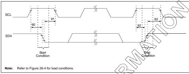
TABLE 26-18: I<sup>2</sup>C™ BUS START/STOP BITS REQUIREMENTS (SLAVE MODE)
