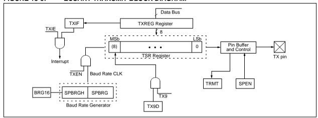
FIGURE 18-4: ASYNCHRONOUS TRANSMISSION
