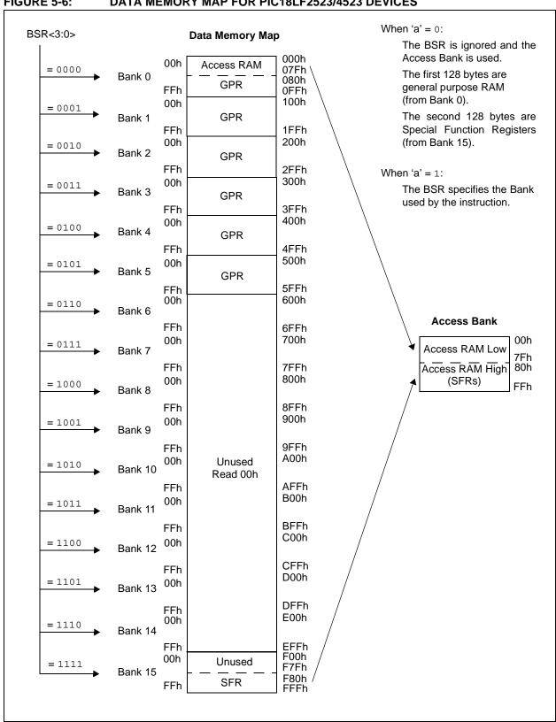
FIGURE 5-6: DATA MEMORY MAP FOR PIC18LF2523/4523 DEVICES
