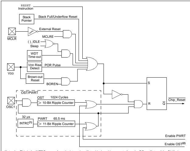
Note 1: This is the INTRC source from the internal oscillator block and is separate from the RC oscillator of the CLKI pin.
