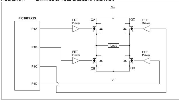
FIGURE 16-7: EXAMPLE OF FULL-BRIDGE APPLICATION
