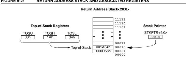
FIGURE 5-2: RETURN ADDRESS STACK AND ASSOCIATED REGISTERS
