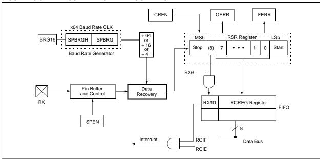
FIGURE 18-7: ASYNCHRONOUS RECEPTION
