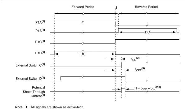
2: t<sub>ON</sub> is the turn-on delay of power switch QC and its driver.
