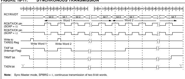
FIGURE 18-12: SYNCHRONOUS TRANSMISSION (THROUGH TXEN)
