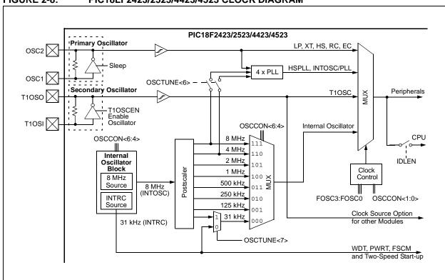
FIGURE 2-8: PIC18LF2423/2523/4423/4523 CLOCK DIAGRAM
