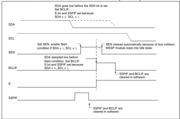
FIGURE 17-29: BUS COLLISION DURING START CONDITION (SCL = 0)
