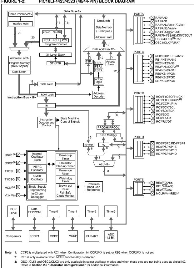
FIGURE 1-2: PIC18LF4423/4523 (40/44-PIN) BLOCK DIAGRAM
