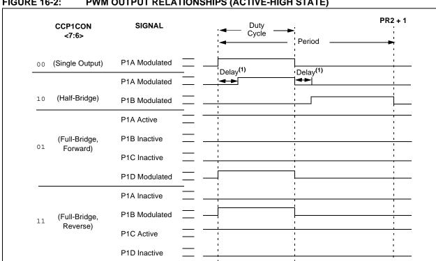
**FIGURE 16-2: PWM OUTPUT RELATIONSHIPS (ACTIVE-HIGH STATE)**
