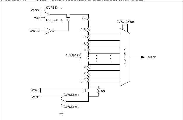
FIGURE 21-1: COMPARATOR VOLTAGE REFERENCE BLOCK DIAGRAM
