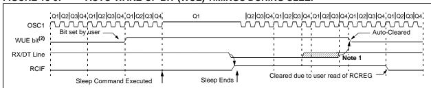
Note 1: If the wake-up event requires long oscillator warm-up time, the auto-clear of the WUE bit can occur before the oscillator is ready. This sequence should not depend on the presence of Q clocks.
