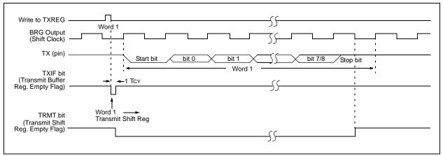
FIGURE 18-5: ASYNCHRONOUS TRANSMISSION (BACK-TO-BACK)
