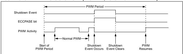
FIGURE 16-10: PWM AUTO-SHUTDOWN (PRSEN = 1, AUTO-RESTART ENABLED)
