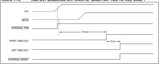
FIGURE 11-7: TIME-OUT SEQUENCE ON POWER-UP (MCLR NOT TIED TO VDD): CASE 2
