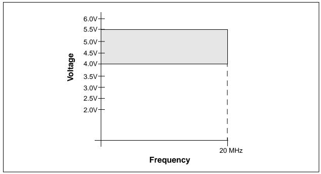
FIGURE 14-2: PIC16LFXXX VOLTAGE-FREQUENCY GRAPH
