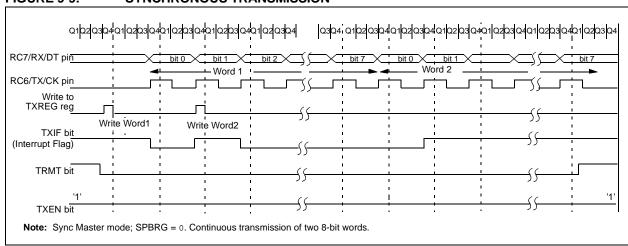
FIGURE 9-10: SYNCHRONOUS TRANSMISSION (THROUGH TXEN)
