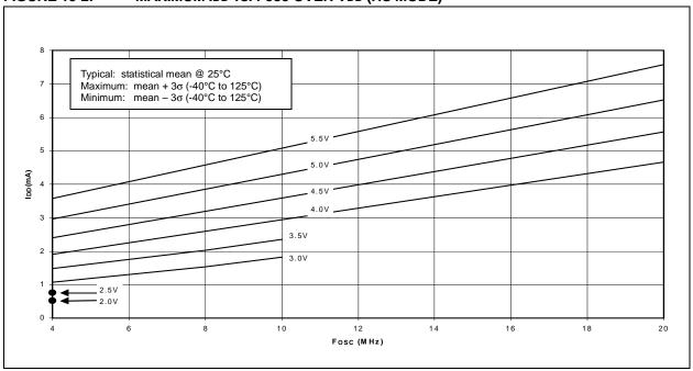
FIGURE 15-3: TYPICAL IDD vs. FOSC OVER VDD (XT MODE)
