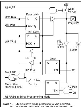
To enable weak pull-ups, set the appropriate TRIS bit(s) and clear the RBPU bit (OPTION\_REG<7>).
