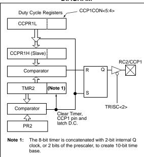
A PWM output (Figure 8-4) has a time base (period) and a time that the output stays high (duty cycle). The frequency of the PWM is the inverse of the period (1/period).
