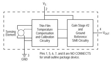
Figure 1. Integrated Pressure Sensor Schematic
