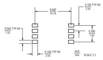
Figure 6. SOP Footprint (Case 482)
