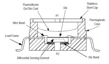
Figure 2. Cross-Sectional Diagram (Not to Scale)
