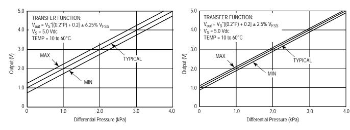
Figure 4. Output vs. Pressure Differential at ±6.25% V<sub>FSS</sub> (without auto zero, Table 1., note 5)
