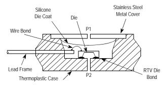
Figure 3. Cross-Sectional Diagrams (not to scale)
