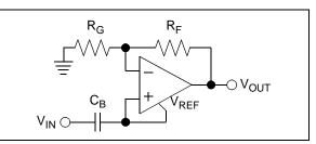
**FIGURE 4-7:** Non-inverting gain circuit using V<sub>REF</sub> (MCP6021 and MCP6023 only).
