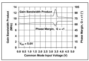
FIGURE 2-23: Gain Bandwidth Product, Phase Margin vs. Common Mode Input Voltage.
