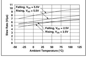
FIGURE 2-25: Slew Rate vs. Temperature.
