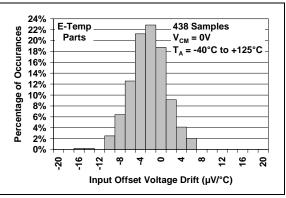
**FIGURE 2-5:** Input Offset Voltage Drift, (Extended Temperature Parts).
