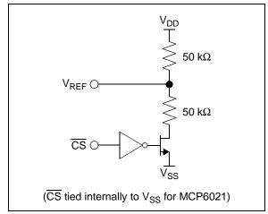
**FIGURE 4-6:** Simplified internal V<sub>REF</sub> circuit (MCP6021 and MCP6023 only).
