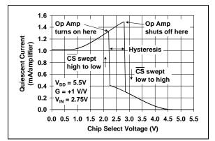
**FIGURE 2-41:** Chip Select ( $\overline{CS}$ ) Hysteresis (MCP6023 only) with  $V_{DD} = 5.5V$ .
