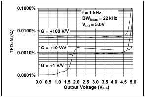
**FIGURE 2-26:** Total Harmonic Distortion plus Noise vs. Output Voltage with f = 1 kHz.
