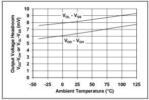
FIGURE 2-34:Output Voltage Headroomvs. Temperature.
