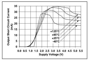
FIGURE 2-15: Output Short-Circuit Current vs. Supply Voltage.
