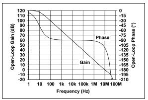
FIGURE 2-18: Open-Loop Gain, Phase vs. Frequency.
