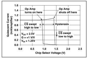
**FIGURE 2-38:** Chip Select ( $\overline{CS}$ ) Hysteresis (MCP6023 only) with  $V_{DD} = 2.5V$ .
