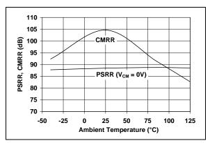
*FIGURE 2-12:* CMRR, PSRR vs. Temperature.
