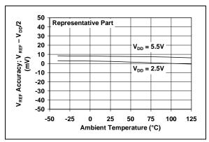
**FIGURE 2-40:** V<sub>REF</sub> Accuracy vs.</sub> Temperature (MCP6021 and MCP6023 only).
