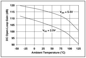
**FIGURE 2-22:** DC Open-Loop Gain vs. Temperature.
