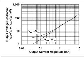
FIGURE 2-31: Output Voltage Headroom vs. Output Current.
