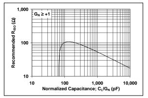
**FIGURE 4-3:** Recommended R<sub>ISO</sub> values for capacitive loads.
