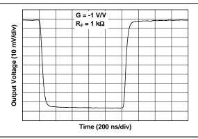
FIGURE 2-35: Small-Signal Inverting Pulse Response.
