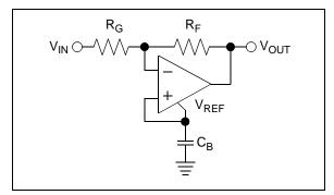
**FIGURE 4-8:** Inverting gain circuit using V<sub>REF</sub> (MCP6021 and MCP6023 only).
