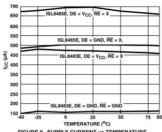
FIGURE 9. SUPPLY CURRENT vs TEMPERATURE
