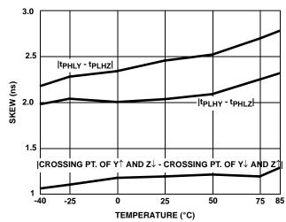
FIGURE 13. DRIVER SKEW vs TEMPERATURE (ISL8485E)
