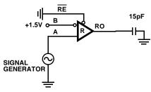
FIGURE 4A. TEST CIRCUIT
