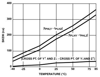
FIGURE 11. DRIVER SKEW vs TEMPERATURE (ISL8483E)
