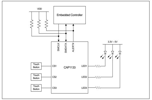
Figure 4.1 System Diagram for CAP1133
