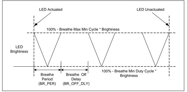
Figure 5.5 Breathe Behavior with Non-Inverted Polarity
