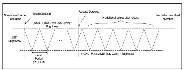
Figure 5.3 Pulse 2 Behavior with Non-Inverted Polarity
