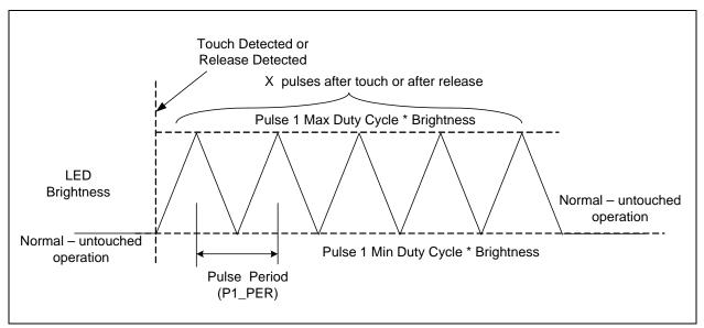
Figure 5.2 Pulse 1 Behavior with Inverted Polarity
