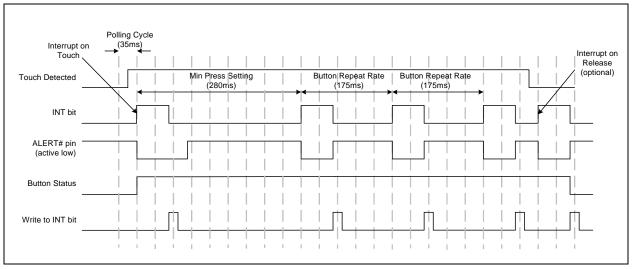
Figure 4.2 Sensor Interrupt Behavior - Repeat Rate Enabled
