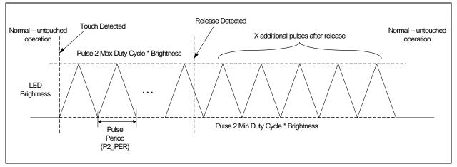
Figure 5.4 Pulse 2 Behavior with Inverted Polarity
