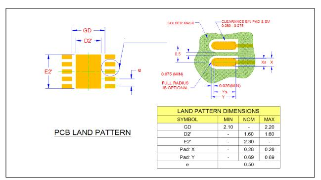
Figure 6.3 10-Pin DFN 3mm x 3mm PCB Footprint
