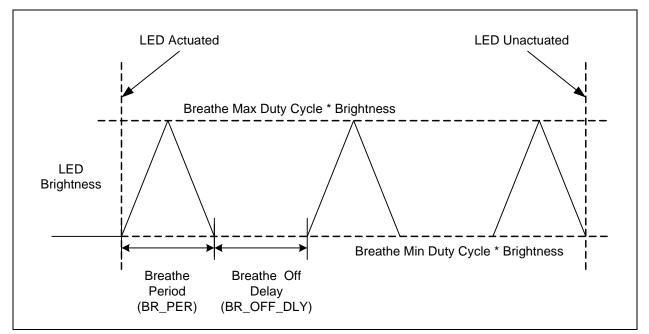
Figure 5.6 Breathe Behavior with Inverted Polarity
