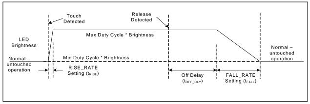
Figure 5.8 Direct Behavior for Inverted Polarity
