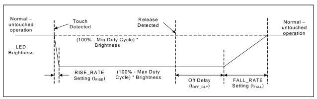
Figure 5.7 Direct Behavior for Non-Inverted Polarity
