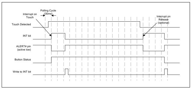
Figure 4.3 Sensor Interrupt Behavior - No Repeat Rate Enabled
