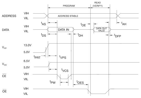
Notes: 1. The input timing reference is 0.8V for  $V_{\parallel L}$  and 2.0V for  $V_{\parallel H}$ .
