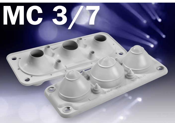
MC 3/7 Multigate is suitable for leading through both low and medium power current cables as well as various types of tubing. It fits directly to a C-standard cut-out (or FL 21).
