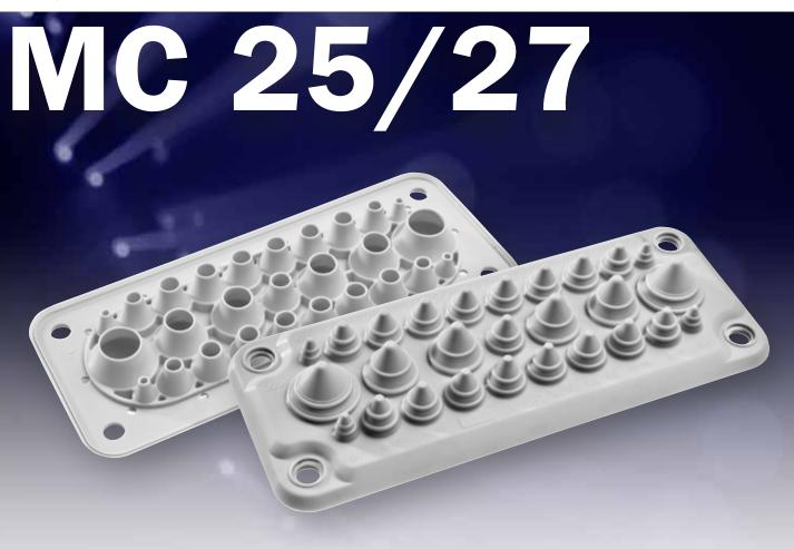
MC 25/27 Multigate is suitable for leading through both low and medium power current cables as well as various types of tubing. It fits directly to a C-standard cut-out (or FL 21).
