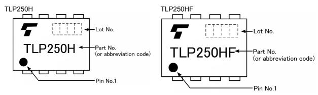
Note: A different marking is used for photocouplers that have been qualified according to option (D4) of EN60747.
