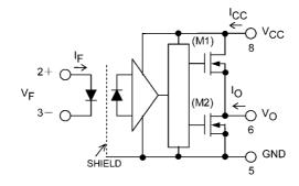
Note: A 0.1- $\mu F$  bypass capacitor must be connected between pin 8 and pin 5.
