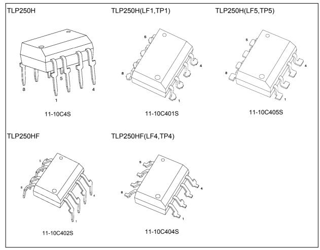
Note: Through-hole type: TLP250H, TLP250HF Lead forming option: (LF1), (LF4), (LF5) Taping option: (TP1), (TP4), (TP5)
