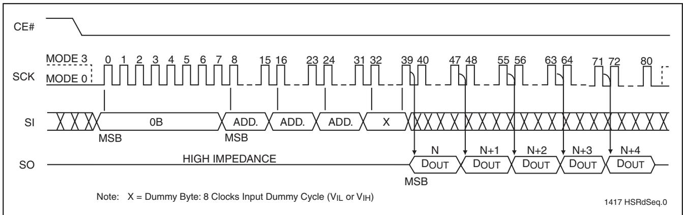
**FIGURE 6: High-Speed-Read Sequence**
