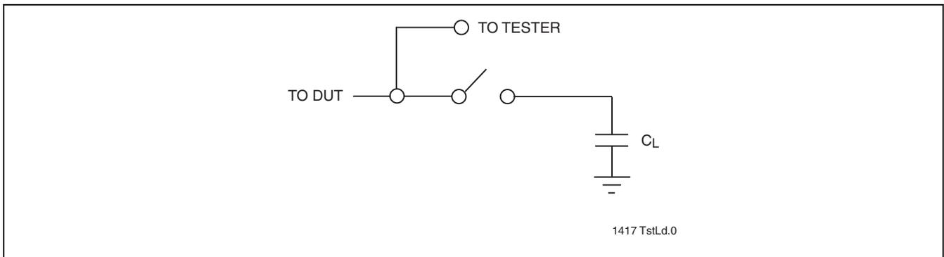
FIGURE 30: A Test Load Example
