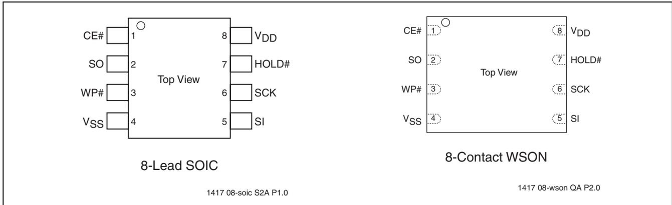
**FIGURE 2: Pin Assignments**
