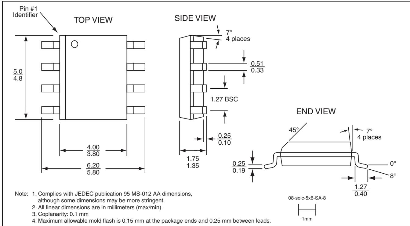
**FIGURE 31: 8-Lead Small Outline Integrated Circuit (SOIC) 150mil Body Width (5mm x 6mm)
