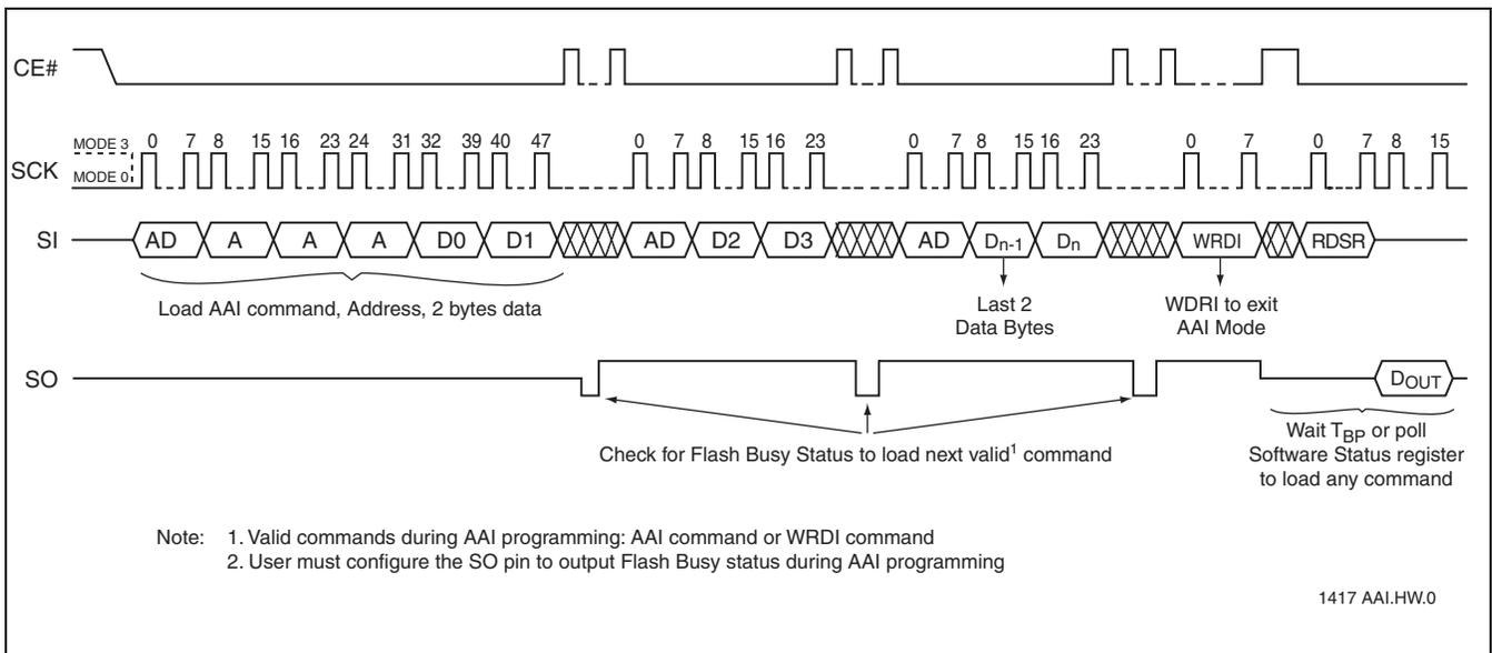
FIGURE 10: Auto Address Increment (AAI) Word-Program Sequence with Hardware End-of-Write Detection
