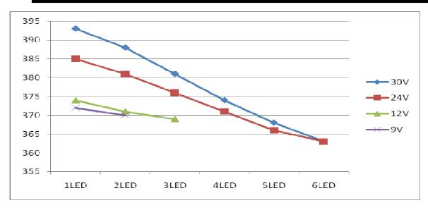
Output current vs. LED cascaded number @L=68uH,  $I_{OUT}$ =370mA
