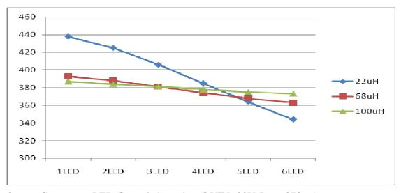
Output Current vs. LED Cascaded number @VIN=30V, I<sub>OUT</sub>=370mA
