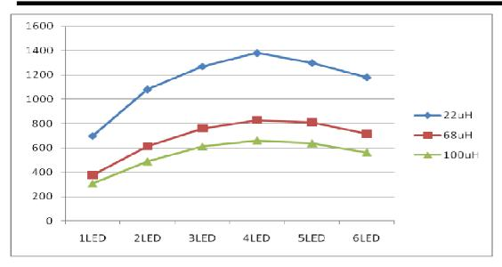
Switching Frequency vs. LED Cascaded Number @VIN=30V, I<sub>OUT</sub>=370mA
