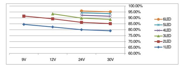
Efficiency vs. input voltage @L=68uH, I<sub>OUT</sub>=770mA
