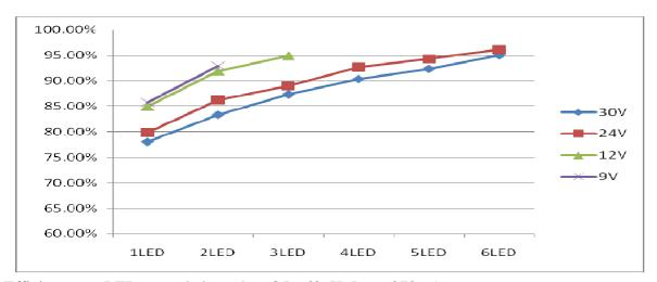
Efficiency vs. LED cascaded number @L=68uH, I<sub>OUT</sub>=370mA
