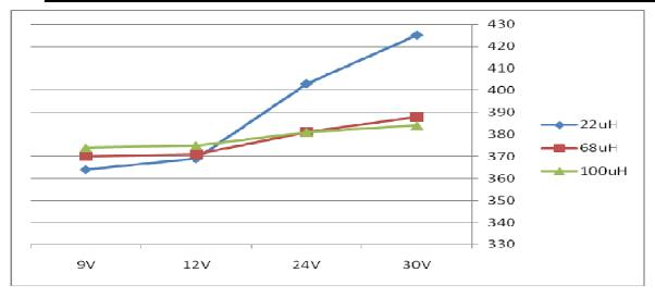
Output current vs. input voltage @2-LED in cascaded, I<sub>OUT</sub>=370mA
