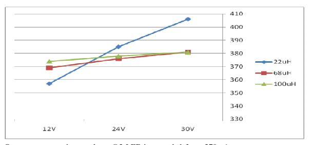
Output current vs. input voltage @3-LED in cascaded, I<sub>OUT</sub>=370mA
