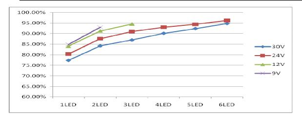
Efficiency vs. LED cascaded number @L=100uH, I<sub>OUT</sub>=370mA
