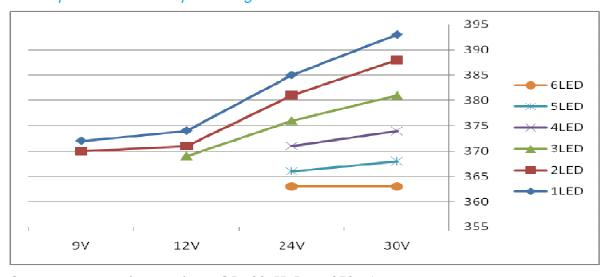
Output current vs. input voltage @L=22uH, I<sub>OUT</sub>=370mA
