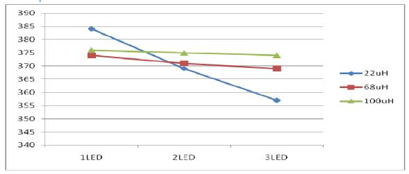
Output Current vs. LED Cascaded number @VIN=12V, I<sub>OUT</sub>=370mA
