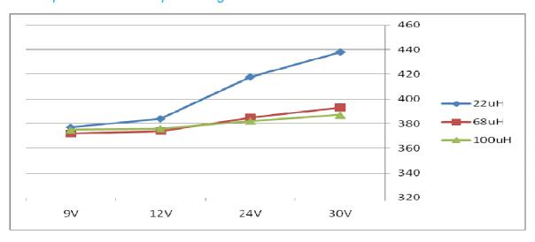
Output current vs. input voltage @1-LED in cascaded, I<sub>OUT</sub>=370mA
