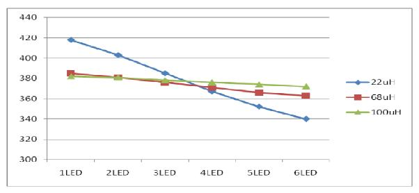
Output Current vs. LED Cascaded number @VIN=24V, I<sub>OUT</sub>=370mA
