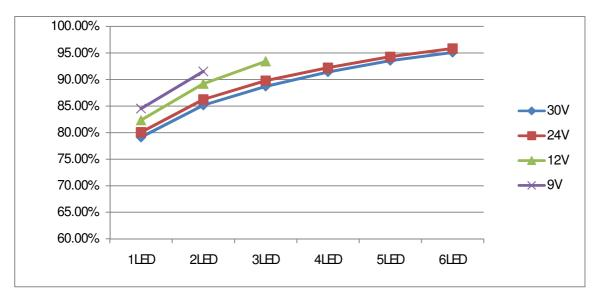
Efficiency vs. LED cascaded number @L=68uH, I<sub>OUT</sub>=770mA
