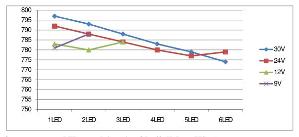
Output current vs. LED cascaded number @L=68uH, I<sub>OUT</sub>=770mA
