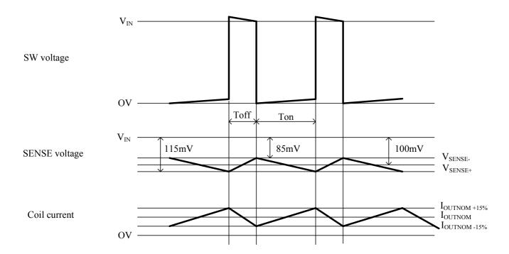
Figure 1-Operating waveforms
