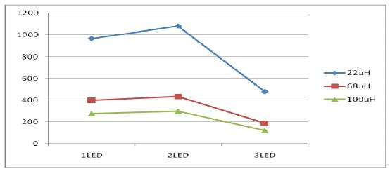
Switching Frequency vs. LED Cascaded Number @VIN=12V, I<sub>OUT</sub>=370mA
