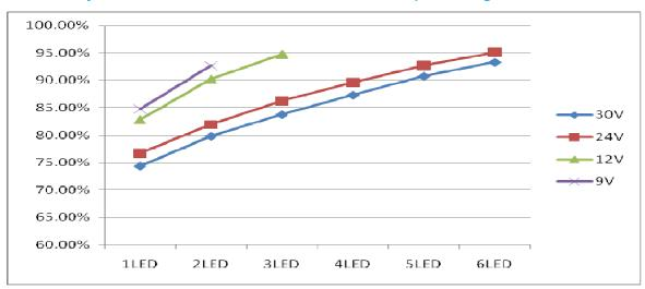
Efficiency vs. LED cascaded number @L=22uH, I<sub>OUT</sub>=370mA
