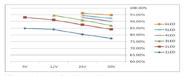
Efficiency vs. input voltage @L=100uH, I<sub>OUT</sub>=370mA
