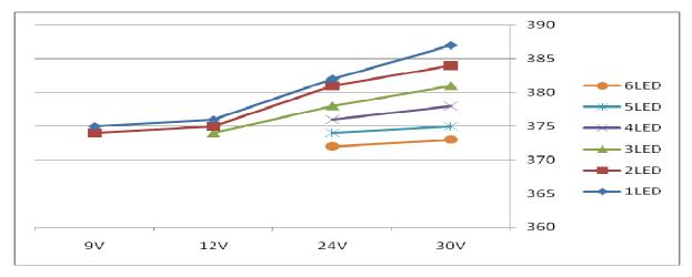
Output current vs. input voltage @L=100uH, I<sub>OUT</sub>=370mA
