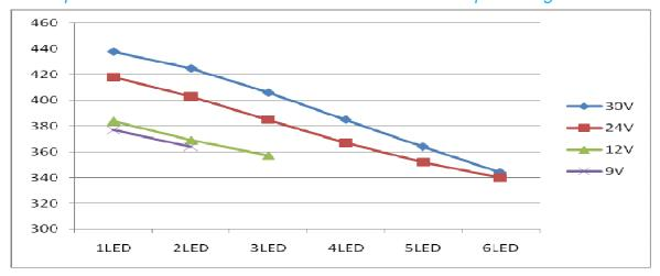
Output current vs. LED cascaded number @L=22uH, I<sub>OUT</sub>=370mA
