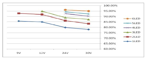
Efficiency vs. input voltage @L=68uH, I<sub>OUT</sub>=370mA
