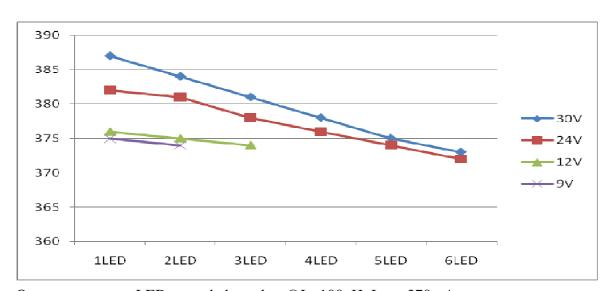
Output current vs. LED cascaded number @L=100uH,  $I_{OUT}$ =370mA
