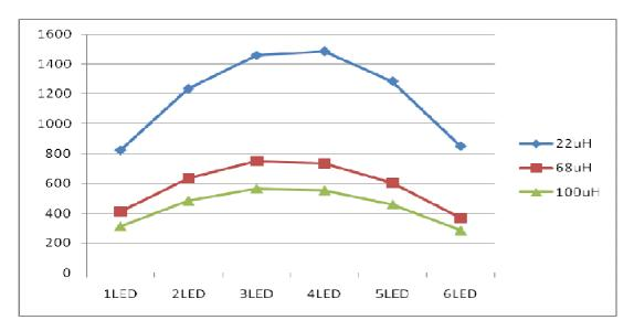
Switching Frequency vs. LED Cascaded Number @VIN=24V, I<sub>OUT</sub>=370mA
