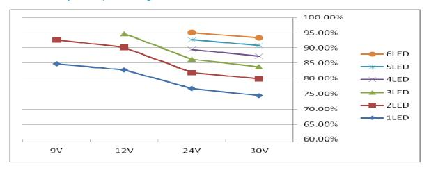
Efficiency vs. input voltage @L=22uH, I<sub>OUT</sub>=370mA
