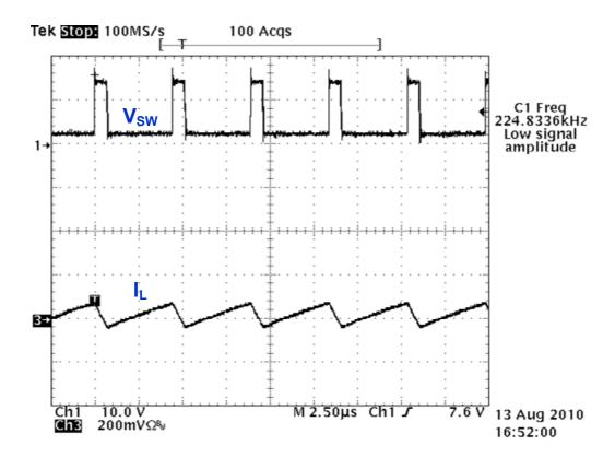
Switching waveform( $V_{IN}=12V$ ,  $R_{SEN}=0.27 \Omega$ , 3-LED)
