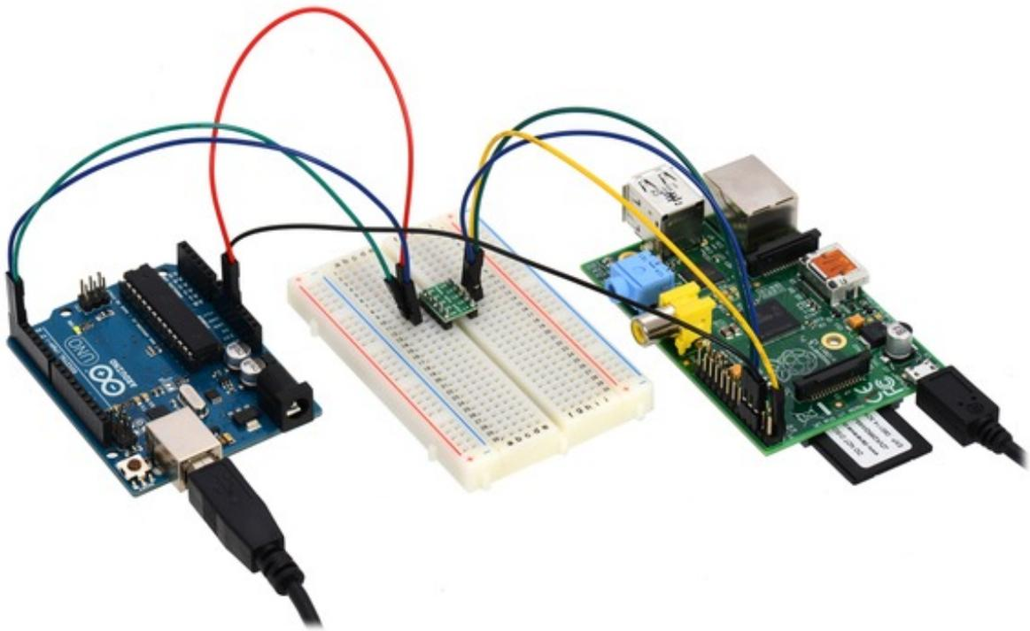
Using the 4-channel bidirectional logic level shifter to create a serial connection between a 5 V Arduino Uno and a 3.3 V Raspberry Pi.
