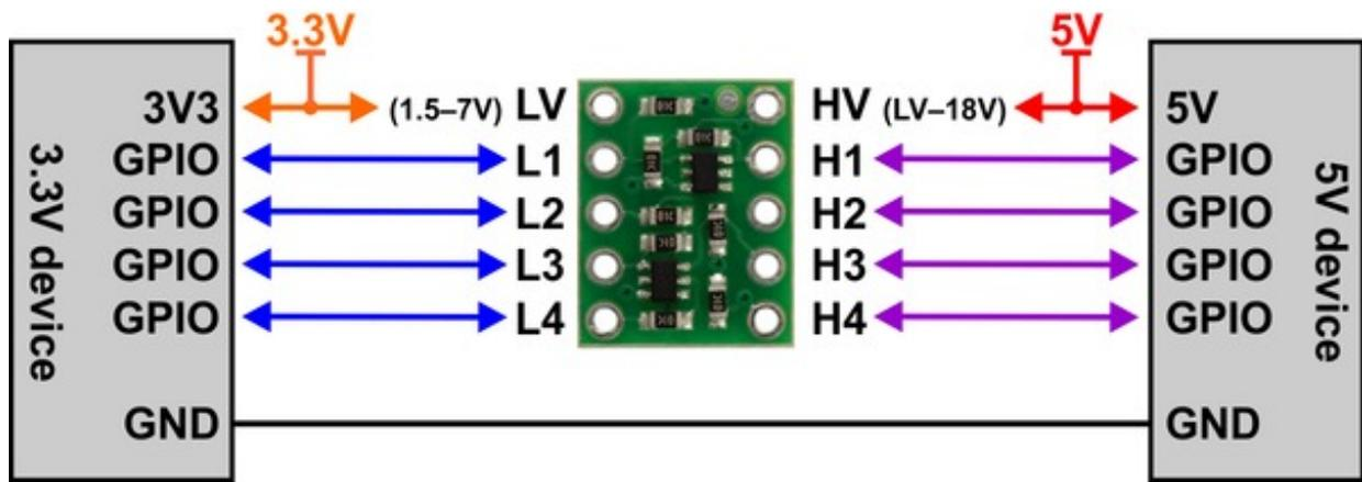
Example wiring diagram for connecting 5 V and 3.3 V devices through the 4-channel bidirectional logic level shifter.
