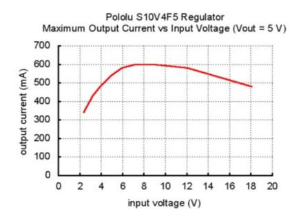
When connecting voltage to electronic circuits, the initial rush of current can cause voltage spikes that are much higher than the input voltage. If these spikes exceed the regulator's maximum voltage, the regulator can be destroyed. In our tests with typical power leads (~30" test clips), input voltages above 11 V caused spikes over 18 V. You can suppress such spikes by soldering a 33  $\mu$ F or larger electrolytic capacitor close to the regulator between VIN and GND.
