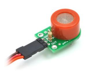
Pololu MQ gas sensor carrier with sensitivitysetting resistor soldered in the horizontal orientation.
