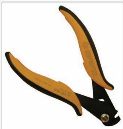
A manual depaneling tool to separate larger sheets of multiple PCB panels in a quick, economic and safe way, leaving well finished cut surfaces; maximum length of the isthmus (tab) must not exceed 2.5 mm.
