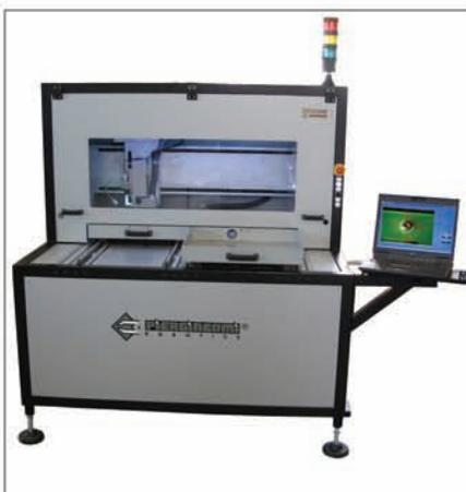
DPA1000 is an automatic depaneling system. Using a vertical milling cutter this system allows to cut isthmus in any direction, following linear or circular lines. DPA1000 functioning is performed by a Personal Computer which manages:
