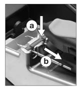
Place the other cartridge in another slot and pull to remove it.
