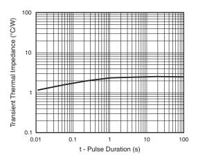
Fig. 6 - Typical Transient Thermal Impedance
