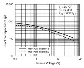
Fig. 5 - Typical Junction Capacitance
