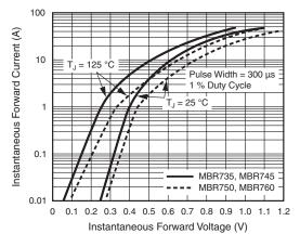
Fig. 3 - Typical Instantaneous Forward Characteristics
