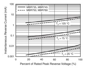
Fig. 4 - Typical Reverse Characteristics
