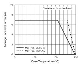
Fig. 1 - Forward Current Derating Curve
