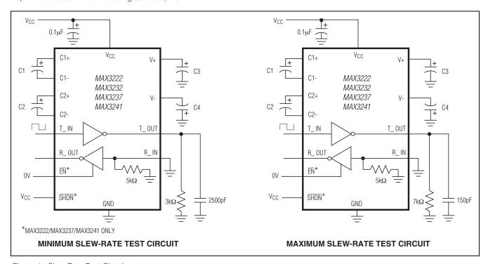
Figure 1. Slew-Rate Test Circuits
