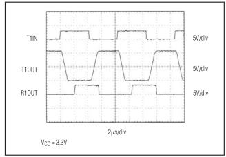
Figure 7. MAX3241 Loopback Test Result at 235kbps
