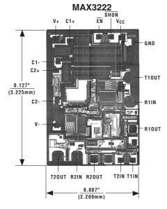
TRANSISTOR COUNT: 339 SUBSTRATE CONNECTED TO GND
