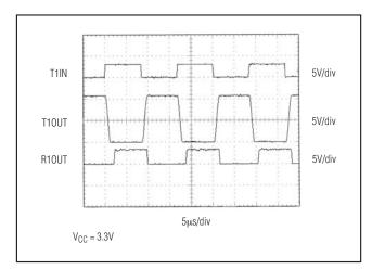
Figure 6. MAX3241 Loopback Test Result at 120kbps
