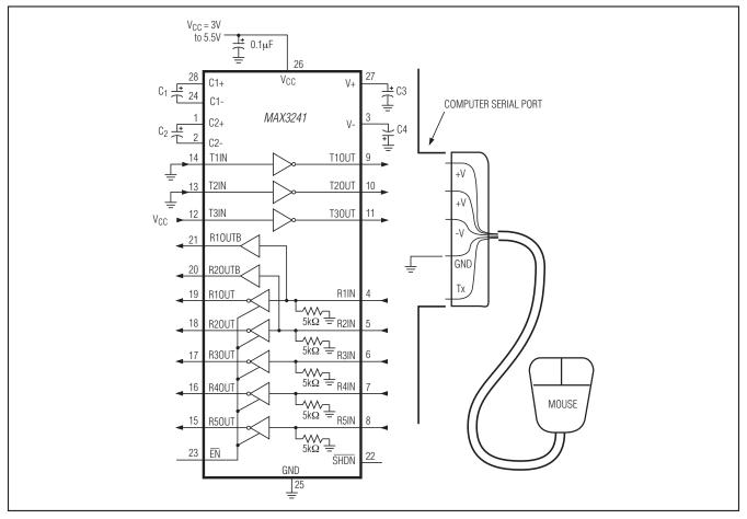
Figure 4b. Mouse Driver Test Circuit
