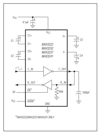
Figure 5. Loopback Test Circuit
