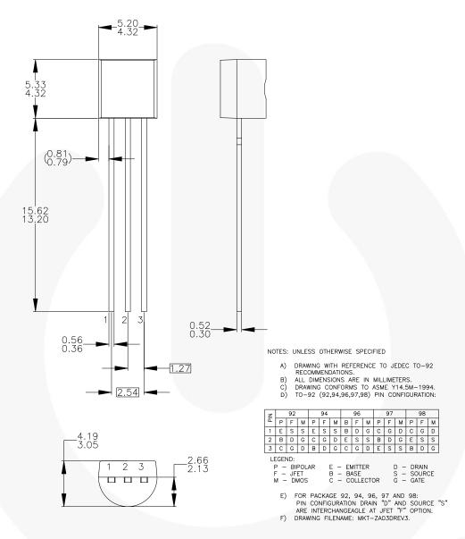
Figure 17. 3-Lead, TO-92, Molded, Standard Straight Lead
