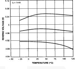
Figure 4. Temperature Drift
