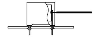
Temperature monitored inside the capacitor.
