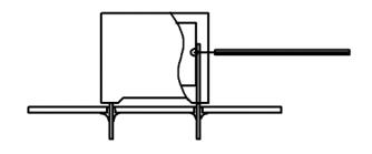
Temperature monitored inside the capacitor.
