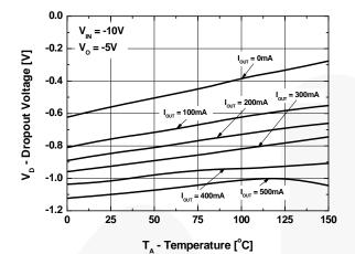
Figure 2. Dropout Voltage
