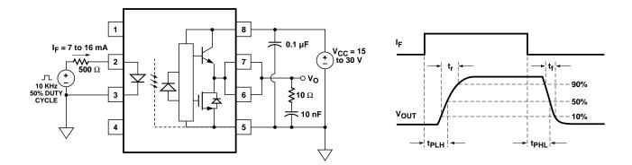
Figure 23.  $t_{PLH},\,t_{PHL},\,t_{r},$  and  $t_{f}\,Test$  Circuit and Waveforms.
