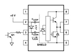
Figure 32. Not Recommended Open Collector Drive Circuit.
