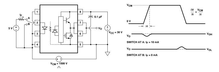
Figure 24. CMR Test Circuit and Waveforms.
