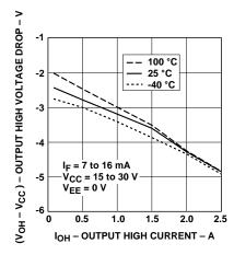
Figure 1.  $\ensuremath{V_{\rm OH}}$  vs. Temperature.
