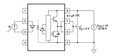
Figure 20.  $V_{OL}$  Test Circuit.
