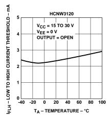
Figure 9. I<sub>FLH</sub> vs. Temperature.
