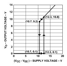
Figure 34. Under Voltage Lock Out.
