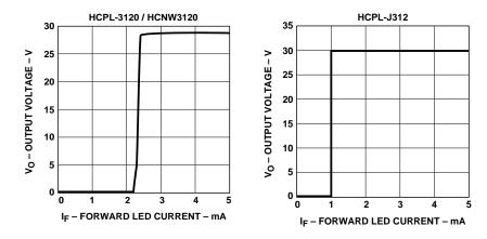
Figure 15. Transfer Characteristics.
