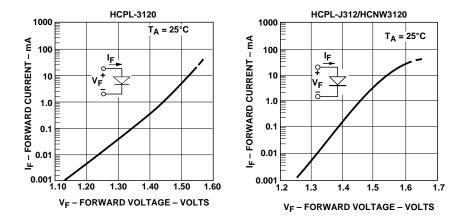
Figure 16. Input Current vs. Forward Voltage.
