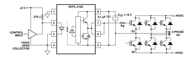
Figure 25. Recommended LED Drive and Application Circuit.
