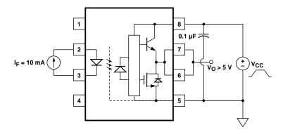
Figure 22. UVLO Test Circuit.
