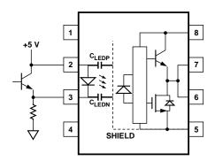
Figure 33. Recommended LED Drive Circuit for Ultra-High CMR.
