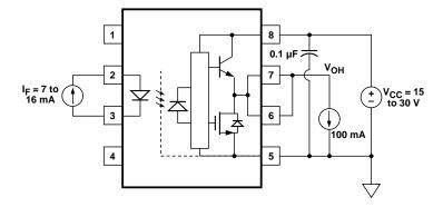
Figure 18.  $I_{OL}$  Test Circuit.
