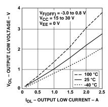
Figure 4.  $V_{OL}$  vs. Temperature.
