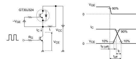
Note 2: Switching loss measurement waveforms
