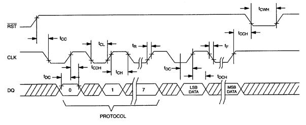
NOTE:  $t_{\text{CL}}$ ,  $t_{\text{CH}}$ ,  $t_{\text{R}}$ , and  $t_{\text{F}}$  apply to both read and write data transfer.
