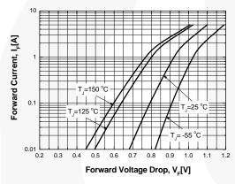
Figure 5. Forward Voltage Characteristics
