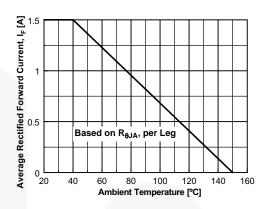
Figure 4. Forward Current Derating Curve
