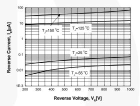
Figure 6. Reverse Current vs. Reverse Voltage
