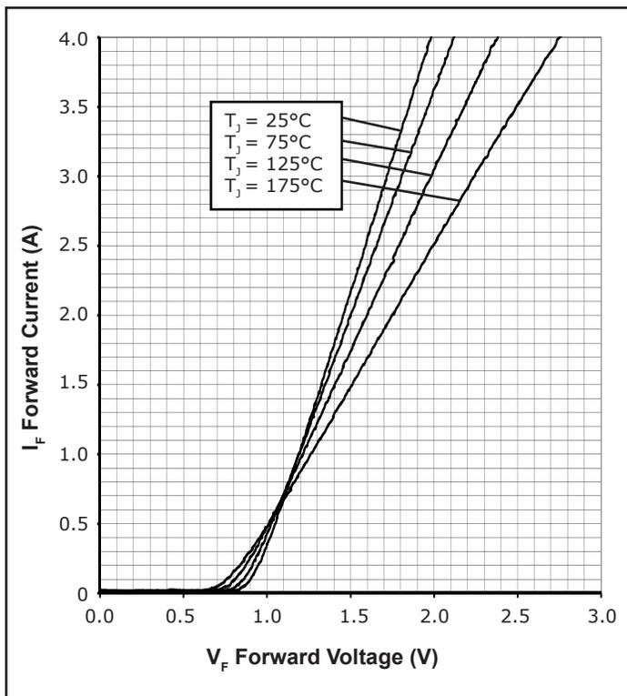
Figure 1. Forward Characteristics
