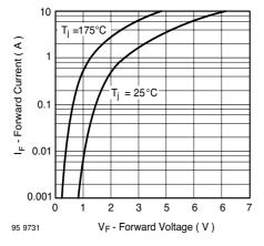
Figure 4. Max. Forward Current vs. Forward Voltage
