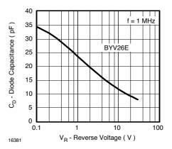
Figure 6. Diode Capacitance vs. Reverse Voltage
