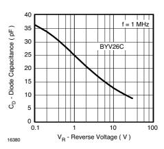
Figure 5. Diode Capacitance vs. Reverse Voltage
