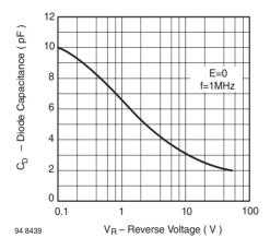
Fig. 5 Diode Capacitance vs. Reverse Voltage
