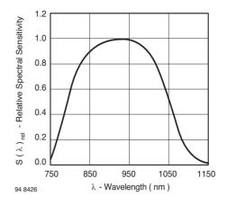
Fig. 6 Relative Spectral Sensitivity vs. Wavelength
