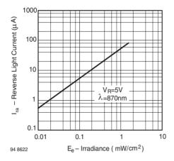
Fig. 3 Reverse Light Current vs. Irradiance
