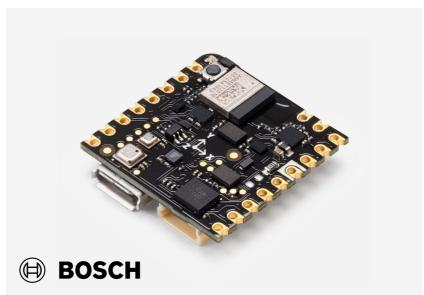
Featuring a 9DoF smart motion sensor and a multi parametric environmental sensor with Al capabilities, the board developed with Bosch Sensortec allows for a wide range of IoT applications. Having Arduino's signature simplicity of integration and scalability, it is also perfect for research projects, rapid
