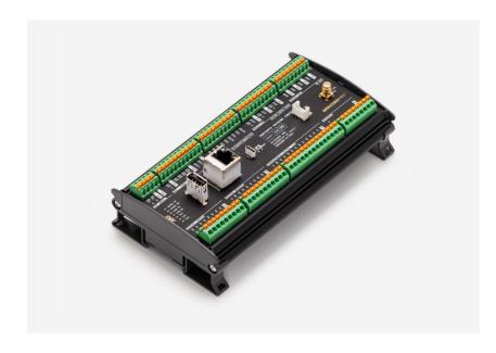
The Portenta Machine Control adds Industrial IoT capabilities to standalone industrial machinery. It enables the collection of real-time data from the factory floor and supports the remote control of equipment, even from the cloud, when desired.
