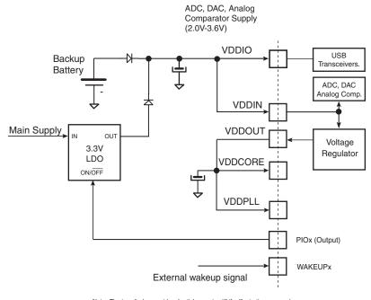
Note: The two diodes provide a "switchover circuit" (for illustration purpose) between the backup battery and the main supply when the system is put in backup mode.
