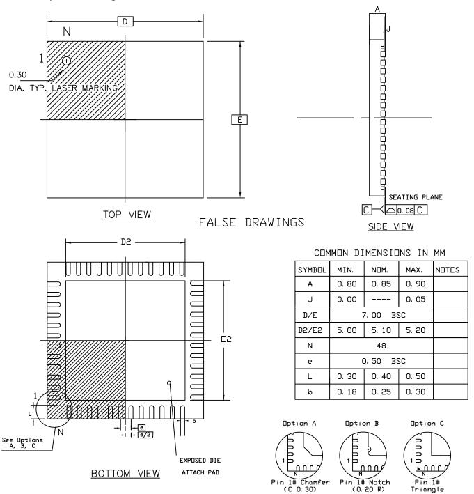
Table 13-3. 48-pad QFN Package Dimensions (in mm)
