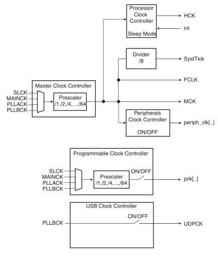
The SysTick calibration value is fixed at 8000 which allows the generation of a time base of 1 ms with SystTick clock at 8 MHz (max HCLK/8 = 64 MHz/8).
