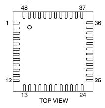
Figure 4-6. Orientation of the 48-lead LQFP Package
