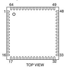
Figure 4-4. Orientation of the 64-lead LQFP Package
