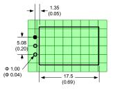
Dimensions are typical values: mm (inch) General Tolerance:  $\pm 0.50 (\pm 0.02)$ Pin Tolerance:  $\pm 0.1 (\pm 0.004)$
