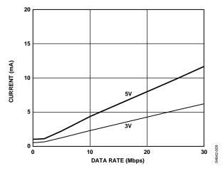
Figure 9. Typical ADuM1200 V<sub>DD1</sub> Supply Current vs. Data Rate for 5 V and 3 V Operation
