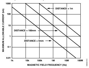
Figure 14. Maximum Allowable Current for Various Current-to-ADuM1200/ADuM1201 Spacings
