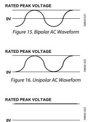
Figure 17. DC Waveform
