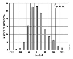
Figure 5. Input Offset Voltage Distribution
