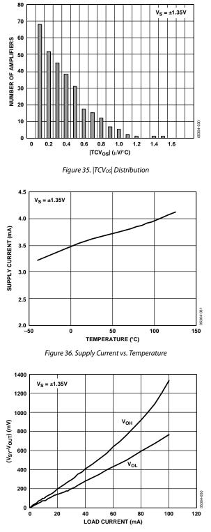
Figure 37. AD8655 Output Voltage to Supply Rail vs. Load Current
