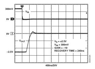
Figure 30. Negative Overload Recovery Time
