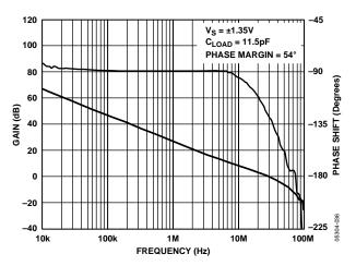
Figure 50. Open-Loop Gain and Phase vs. Frequency
