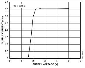
Figure 10. Supply Current vs. Supply Voltage
