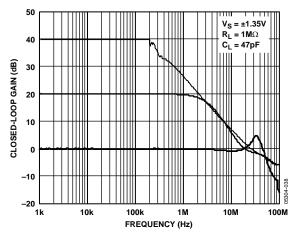
Figure 52. Closed-Loop Gain vs. Frequency
