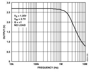
Figure 53. Maximum Output Swing vs. Frequency
