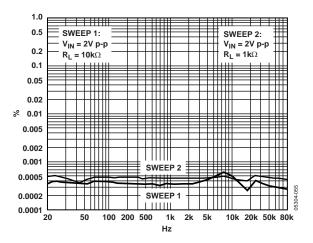
Figure 60. THD + Noise vs. Frequency
