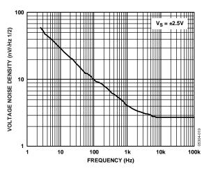
Figure 20. Voltage Noise Density vs. Frequency
