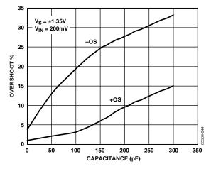
Figure 44. Small Signal Overshoot vs. Load Capacitance
