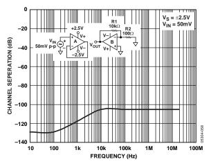
Figure 55. Channel Separation vs. Frequency
