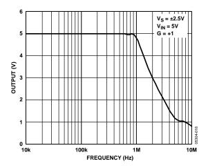
Figure 26. Maximum Output Swing vs. Frequency
