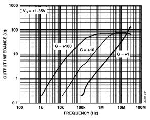
Figure 54. Output Impedance vs. Frequency
