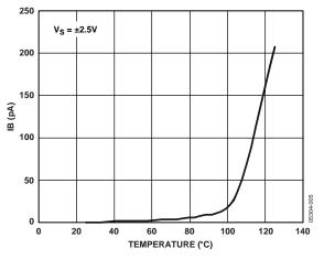
Figure 9. Input Bias Current vs. Temperature
