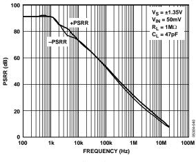
Figure 49. Small Signal PSSR vs. Frequency
