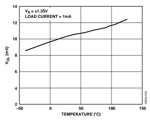
Figure 40. Output Voltage Swing Low vs. Temperature
