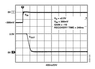
Figure 31. Positive Overload Recovery Time
