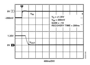
Figure 46. Positive Overload Recovery Time
