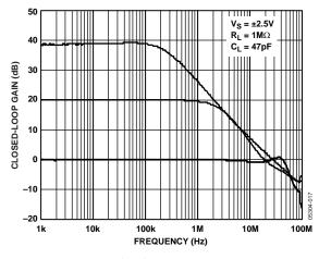
Figure 25. Closed-Loop Gain vs. Frequency
