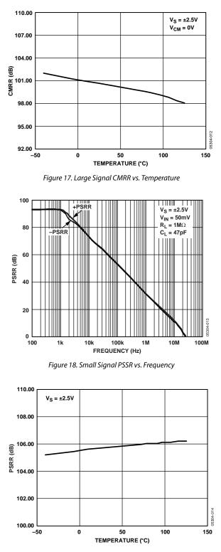
Figure 19. Large Signal PSSR vs. Temperature
