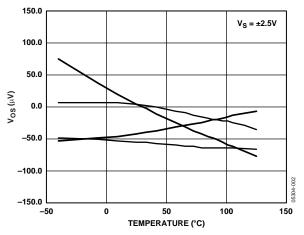
Figure 6. Input Offset Voltage vs. Temperature
