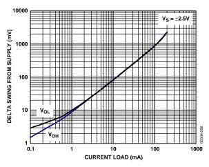
Figure 13. AD8656 Output Swing vs. Current Load
