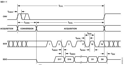
Figure 38. 3-Wire CS Mode with Busy Indicator Serial Interface Timing (SDI High)
