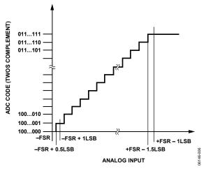
Figure 28. ADC Ideal Transfer Function
