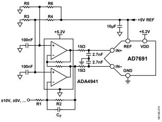
Figure 32. Single-Ended-to-Differential Driver Circuit
