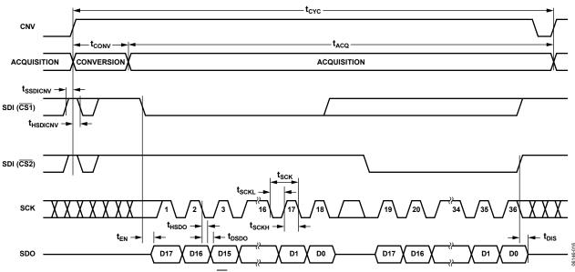
Figure 40. 4-Wire CS Mode Without Busy Indicator Serial Interface Timing
