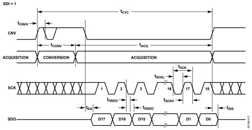
Figure 36. 3-Wire CS Mode Without Busy Indicator Serial Interface Timing (SDI High)
