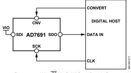
Figure 35. 3-Wire CS Mode Without Busy Indicator Connection Diagram (SDI High)
