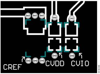
Figure 48. Example Layout of the AD7691 (Bottom Layer)
