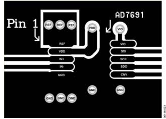
Figure 47. Example Layout of the AD7691 (Top Layer)
