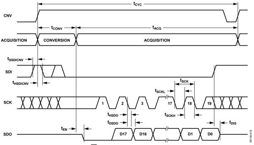
Figure 42. 4-Wire  $\overline{\mathsf{CS}}$  Mode with Busy Indicator Serial Interface Timing
