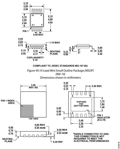
Figure 50. 10-Lead Lead Frame Chip Scale Package [QFN (LFCSP\_WD)] 3 mm × 3 mm Body, Very Very Thin, Dual Lead (CP-10-9) Dimensions shown in millimeters
