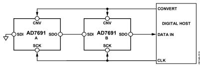
Figure 43. Chain Mode Without Busy Indicator Connection Diagram
