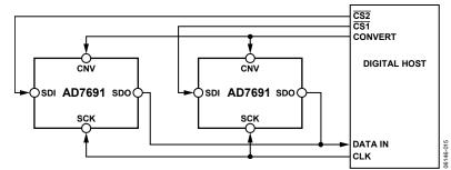
Figure 39. 4-Wire  $\overline{CS}$  Mode Without Busy Indicator Connection Diagram
