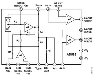
Figure 3. AD588 Functional Block Diagram
