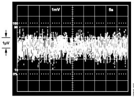
Figure 7. 0.1 Hz to 10 Hz Noise (0.1 Hz to 10 Hz BPF with Gain of 1000 Applied)
