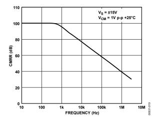
Figure 19. Common-Mode Rejection vs. Frequency (A3, A4)
