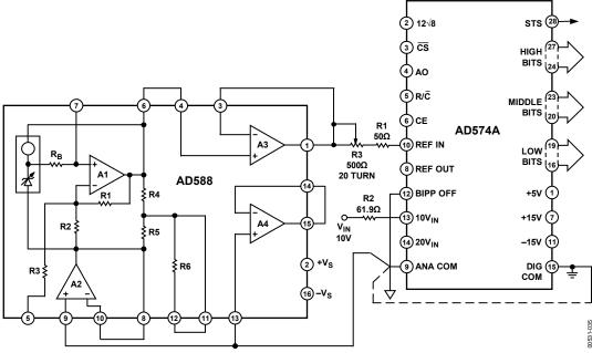
Figure 35. AD588/AD574A Connections
