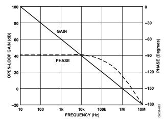
Figure 15. Open-Loop Frequency Response (A3, A4)
