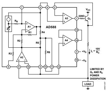
Figure 37. Boosted Precision Current Source
