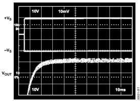
Figure 11. Turn-On with  $CN = 1 \mu F$
