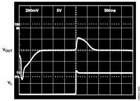
Figure 22. Large-Scale Transient Response
