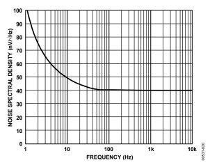
Figure 20. Input Noise Voltage Spectral Density
