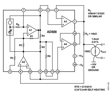
Figure 36. Precision Current Source for RTD
