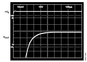
Figure 9. Electrical Turn-On
