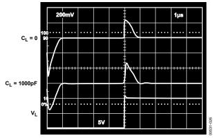
Figure 26. Output Response with Capacitive Load
