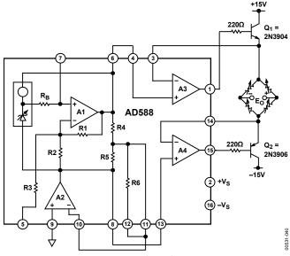
Figure 40. Bipolar Bridge Drive
