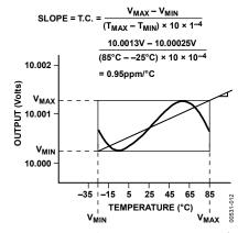
Figure 12. Typical AD588BQ Temperature Drift
