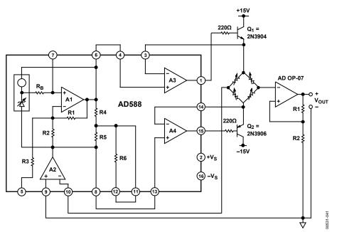
Figure 41. Floating Bipolar Bridge Drive with Minimum CMV
