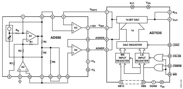
Figure 32. AD588/AD7535 Connections
