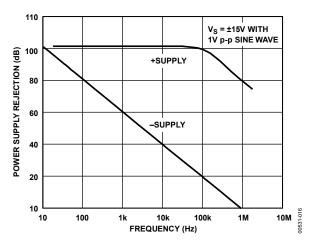
Figure 16. Power Supply Rejection vs. Frequency (A3, A4)
