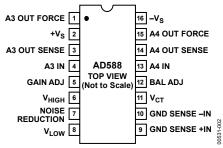
Figure 2. Pin Configuration
