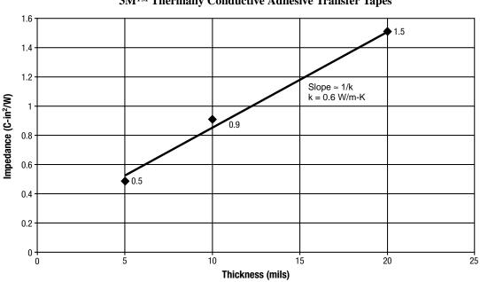
3M<sup>™</sup> Thermally Conductive Adhesive Transfer Tapes
