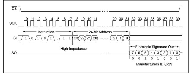
Driving  $\overline{CS}$  high after the 8-bit RDID command, but before the Electronic Signature has been transmitted, will still ensure the device will be taken out of Deep Power-Down mode. However, there is a delay  $T_{REL}$  that occurs before the device returns to Standby mode ( $I_{CCS}$ ), as shown in Figure 2-13.
