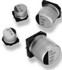
Tyco Electronics vertical chip-type aluminum electrolytic capacitors are designed for surface mounting in high density PCB population. Supplied on tape and reel for use with automatic placement equipment. The TYEH series offers miniature case sizes with an extended temperature range (-40°C to +105°C) and voltage ratings up to 100V dc. Suitable for applications requiring reliability under more demanding conditions.
