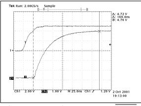
**FIGURE 2-7:** CLEAR pin high to ALERT pin high Timing Diagram.
