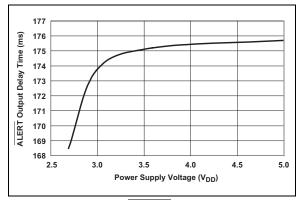
FIGURE 2-6: ALERT Output Delay vs. Power Supply Voltage.
