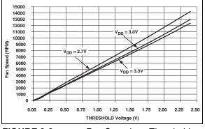
FIGURE 2-2: Fan Speed vs. Threshold Voltage.
