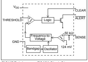
FIGURE 4-1: TC670 Block Diagram.
