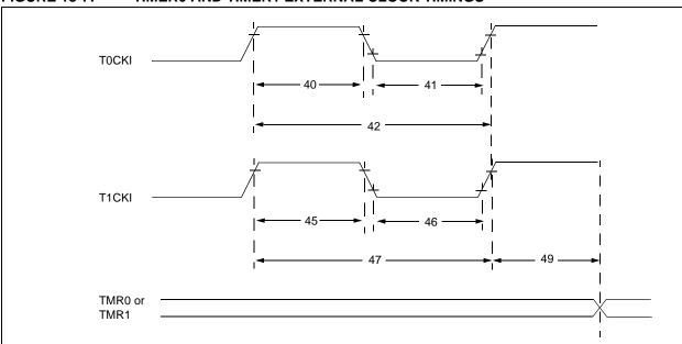
FIGURE 18-7: TIMERO AND TIMER1 EXTERNAL CLOCK TIMINGS
