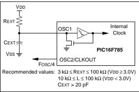
In RCIO mode, the RC circuit is connected to the OSC1 pin. The OSC2 pin becomes an additional general purpose I/O pin. The I/O pin becomes bit 4 of PORTA (RA4). Figure 3-6 shows the RCIO mode connections.
