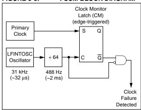
The FSCM function is enabled by setting the FCMEN bit in Configuration Word (CONFIG). It is applicable to all external clock options (LP, XT, HS, EC, RC or I/O modes).
