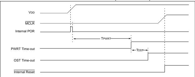
FIGURE 15-5: TIME-OUT SEQUENCE ON POWER-UP (MCLR WITH VDD)
