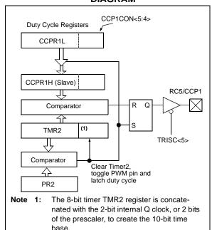
The PWM output (Figure 8-4) has a time base (period) and a time that the output stays high (duty cycle). The frequency of the PWM is the inverse of the period (1/period).
