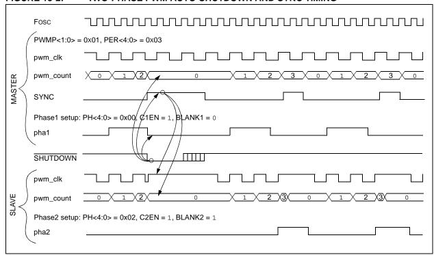
FIGURE 13-3: TWO-PHASE PWM START-UP TIMING
