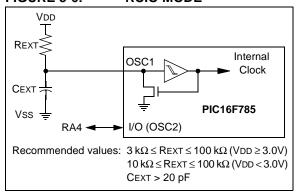
The RC oscillator frequency is a function of the supply voltage, the resistor (REXT) and capacitor (CEXT) values and the operating temperature. In addition to this, the oscillator frequency will vary from unit-to-unit due to normal threshold voltage. Furthermore, the difference in lead frame capacitance between package types will also affect the oscillation frequency or low CEXT values. The user also needs to take into account variation due to tolerance of external RC components used.
