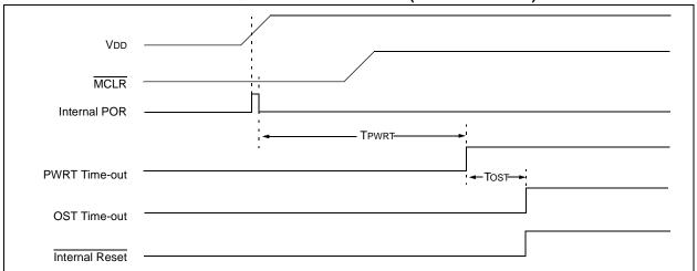
FIGURE 15-4: TIME-OUT SEQUENCE ON POWER-UP (DELAYED MCLR): CASE 2
