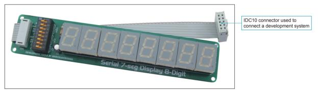
Figure 1: Serial 7-Seg Display 8-Digit additional board
