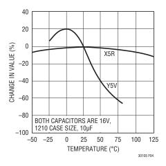
Figure 4. Ceramic Capacitor Temperature Characteristics
