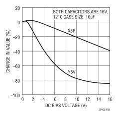
Figure 3. Ceramic Capacitor DC Bias Characteristics
