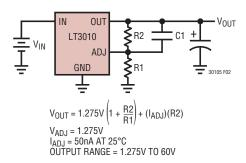
Figure 2. Adjustable Operation
