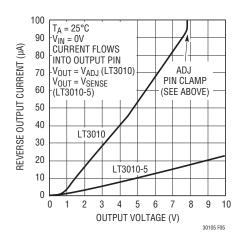
Figure 5. Reverse Output Current
