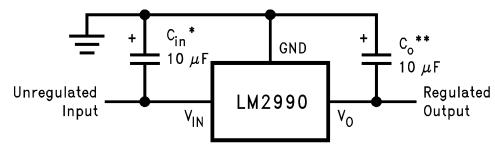
\*Required if the regulator is located further than 6 inches from the power supply filter capacitors. A 1  $\mu$ F solid tantalum or a 10  $\mu$ F aluminum electrolytic capacitor is recommended.
