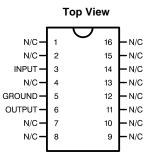
Figure 4. 16-Lead CDIP Package See Package Number NFE0016A
