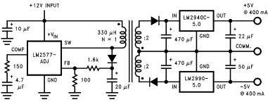
Figure 25. Post Regulator for an Isolated Switching Power Supply
