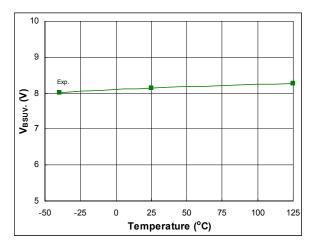
Figure 55: V<sub>BSUV-</sub> vs. temperature
