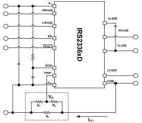
Figure 14: Programming the over-current protection
