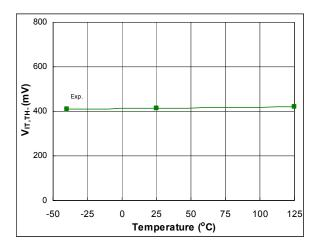
Figure 57: VIT,TH- vs. temperature
