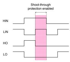
Figure 10: Illustration of shoot-through protection circuitry
