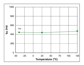
Figure 43: t<sub>EN</sub> vs. temperature
