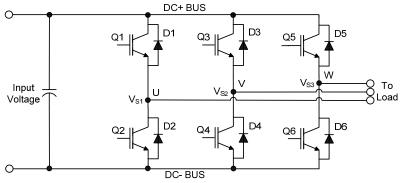
Figure 25: Three phase inverter
