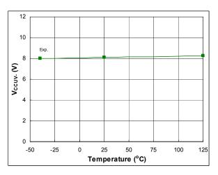
Figure 53: V<sub>CCUV-</sub> vs. temperature
