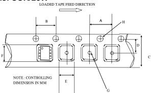
CARRIER TAPE DIMENSION FOR 28SOICW
