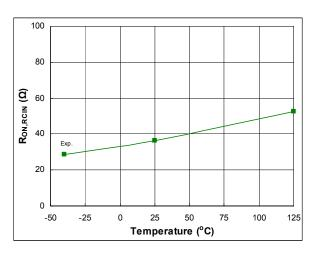
Figure 58: R<sub>ON,RCIN</sub> vs. temperature
