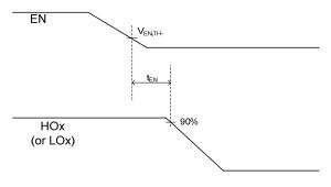
Figure 11: Output enable timing waveform
