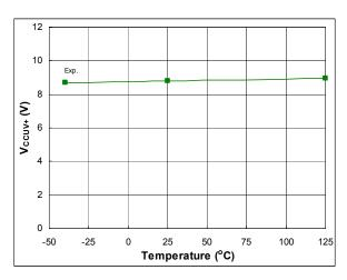
Figure 52: V<sub>CCUV+</sub> vs. temperature
