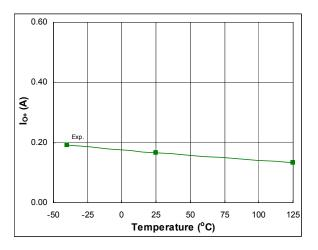
Figure 50: I<sub>0+</sub> vs. temperature
