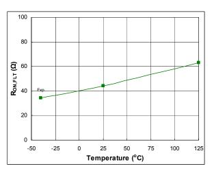
Figure 59: R<sub>ON,FLT</sub> vs. temperature
