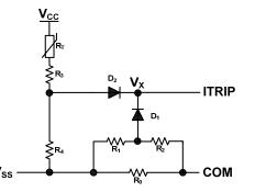
Figure 15: Programming over-temperature protection
