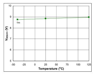
Figure 54: V<sub>BSUV+</sub> vs. temperature
