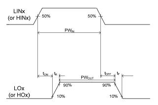
Figure 3: Switching time waveforms (IRS2336(D))
