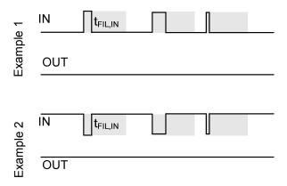
Figure 19: Noise rejecting input filters
