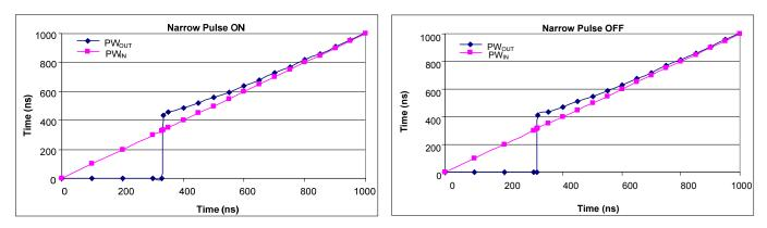
Figure 20: IRS2336xD input filter characteristic
