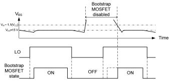
Figure 22: Internal bootstrap MOSFET connection
