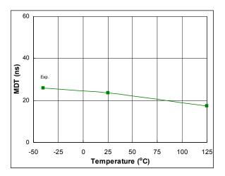
Figure 45: MDT vs. temperature
