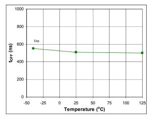
Figure 39: t<sub>OFF</sub> vs. temperature
