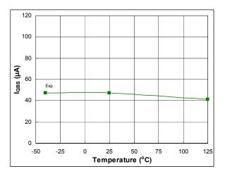
Figure 49: IQBS vs. temperature
