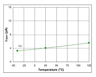
Figure 47: I<sub>ITRIP+</sub> vs. temperature
