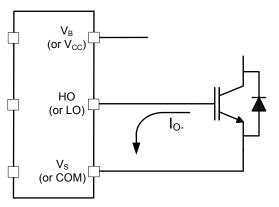
Figure 2: HVIC sinking current
