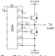
Figure 37: V<sub>s</sub> clamping diode
