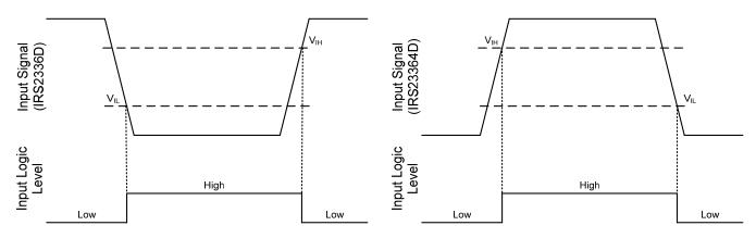
Figure 8: HIN & LIN input thresholds
