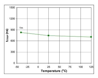
Figure 41: t<sub>ITRIP</sub> vs. temperature
