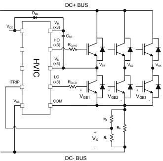
Figure 24: Separate V<sub>ss</sub> and COM pins
