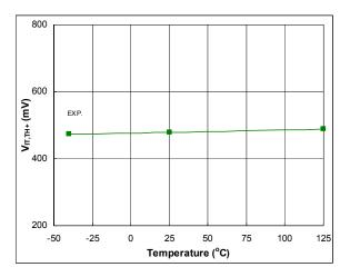
Figure 56: VIT,TH+ vs. temperature
