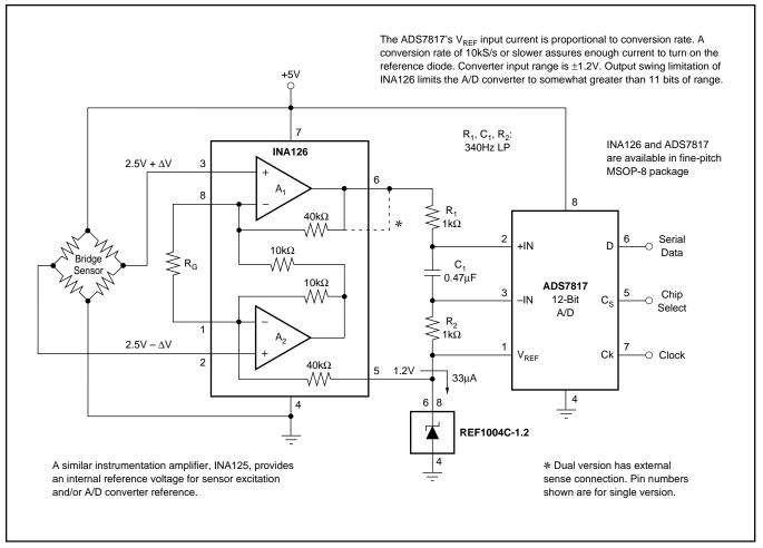
FIGURE 4. Bridge Signal Acquisition—Single 5V Supply.
