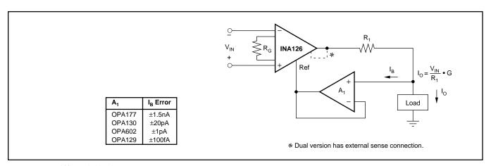
FIGURE 5. Differential Voltage-to-Current Converter.
