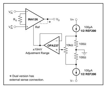
FIGURE 2. Optional Trimming of Output Offset Voltage.
