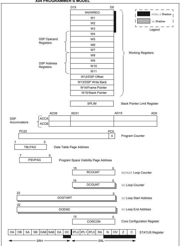
FIGURE 2-2: dsPIC33FJ32GP302/304, dsPIC33FJ64GPX02/X04, AND dsPIC33FJ128GPX02/ X04 PROGRAMMER'S MODEL
