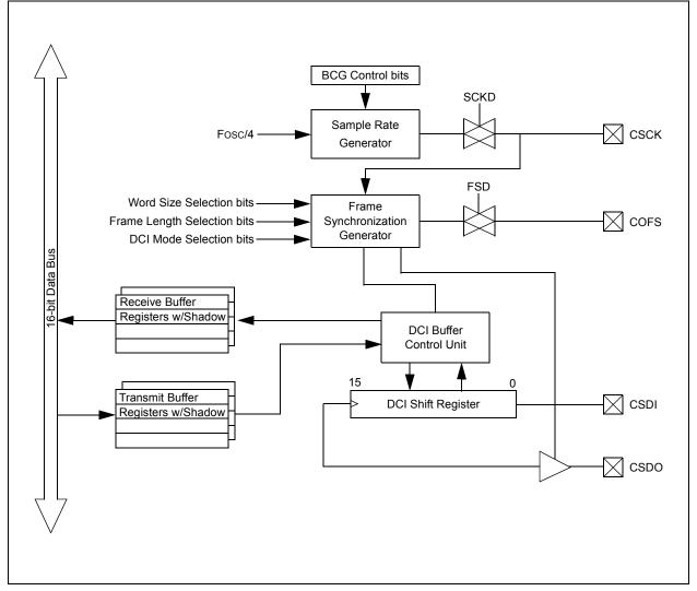
FIGURE 19-1: DCI MODULE BLOCK DIAGRAM
