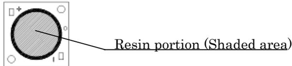
3. This product should be secured firmly by fastening an M3 screw on both sides of the product. Please be careful not to apply any stress to the product during the clamping operation. As the connection status could vary depending on materials of outer heat sink, please check thoroughly.
