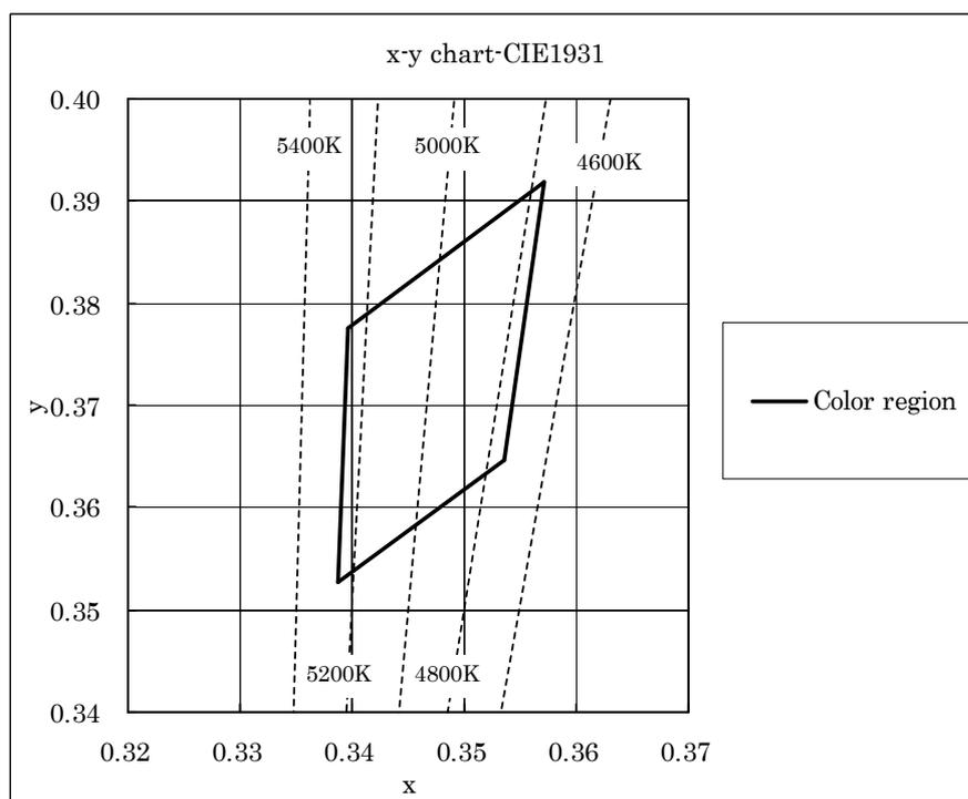
Note: The tolerance of measurement at our tester is V<sub>F</sub>+/-3%, Φ<sub>v</sub>+/-10%, Chromaticity(x,y)+/-0.005 and Ra+/-1.
