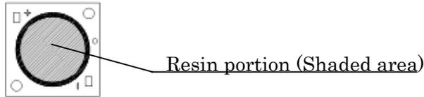
3. This product should be secured firmly by fastening an M3 screw on both sides of the product. Please be careful not to apply any stress to the product during the clamping operation. As the connection status could vary depending on materials of outer heat sink, please check thoroughly.
